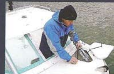
A hatch gives access to the anchor locker
